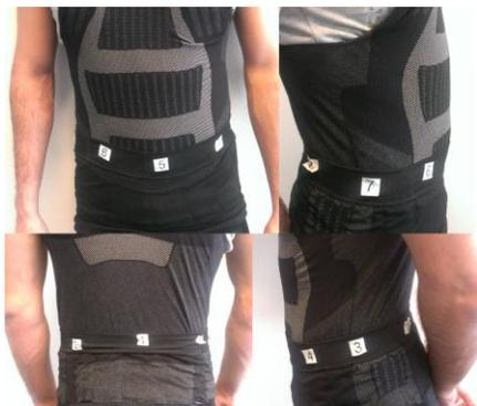
**Figure 5: The GuideBelt prototype, built using 8 phones (Nexus 5), arranged in fixed and precise positions.**
