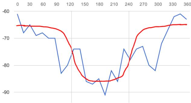
**Figure 2: Graph showing the RSSI log of the rotation from the conducted experiment. As can be the signal strength begins starts to reduce drastically from 120° and goes to a trough and begins to rise significantly again from 240°, considering a margin of error of 10°.**
